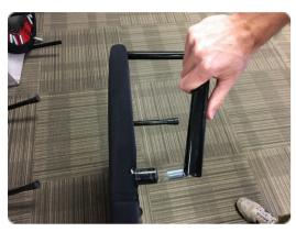
Step 2: Carefully bend the leg 90 degrees so that the inner leg-spring goes between the cylinder leg.
