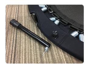
Step 3: Unhook and remove the leg.
