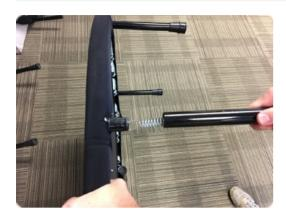
Step 1: Pull cylinder leg off the stud to expose the inner leg-spring.
