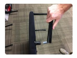
Step 2: Carefully bend the leg 90 degrees so that the inner leg-spring goes between the cylinder leg.
